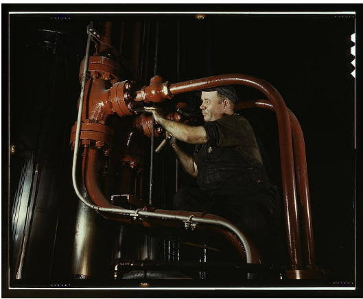
Maintenance man at the Combustion Engineering Co. working at the largest cold steel hydraulic press in the world, Chattanooga, Tenn. This press can shape steel plates several inches in thickness [1942]
